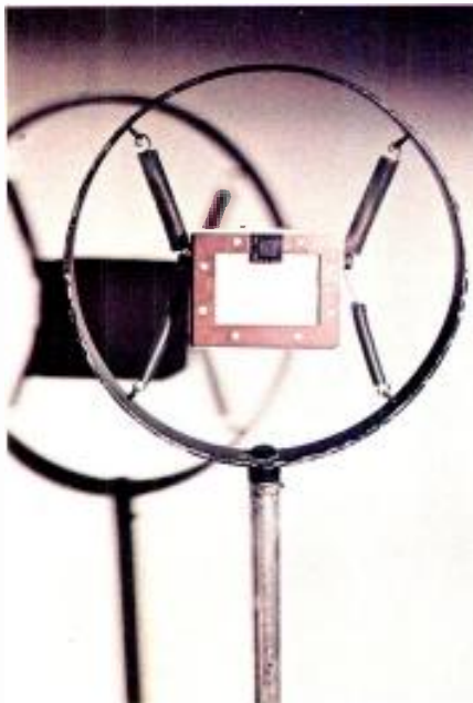
Telefunken "Reisz" microphone, circa 1930, carbon-type, in solid marble housing, 50-6 kHz. (Photo courtesy of AEG-Telefunken Archives and Ampex Museum.)
