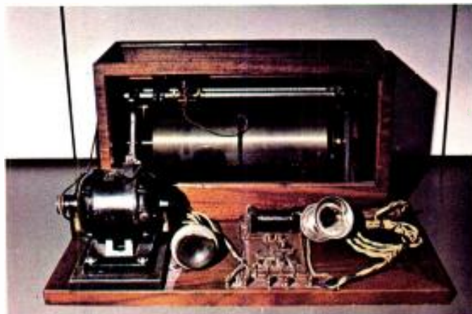
Poulsen Telegraphone, complete (1899). Poulsen intended this device—record/PB time = 30 seconds—to be an automatic telephone answering machine. (Photo courtesy of the Deutsches Museum, Munich.)
