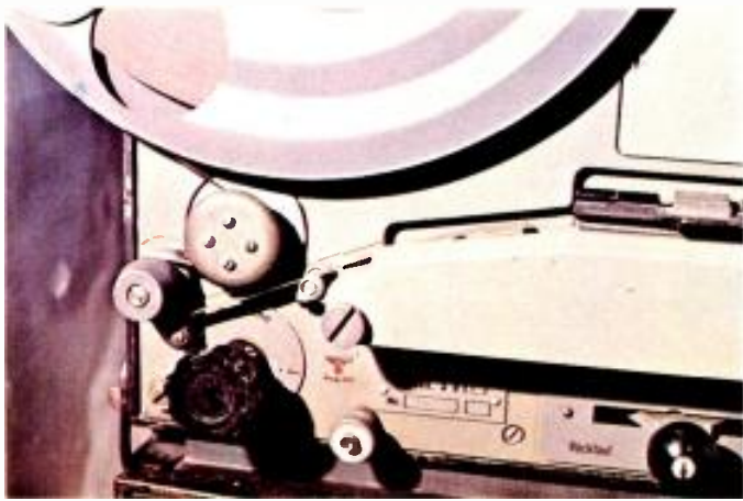
Spinning head (4 gaps, 90 degrees to tape path) of Tonschreiber "Berta"; made by AEG, Berlin, circa 1939. (Photo courtesy of AEG—Telefunken and Ampex.)
