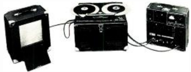
An AEG Magnetophon K-4, circa 1938. The DC bias version had a frequency response of 50-6 kHz, 5 percent distortion and a dynamic range of 40 dB. Once modified with Walter Weber's AC record bias, the frequency response improved to 40-15 kHz, with a 65 dB dynamic range and less than 3 percent distortion. (Photo courtesy of the AEG-Telefunken Archives, Braunschweig, Germany.)
